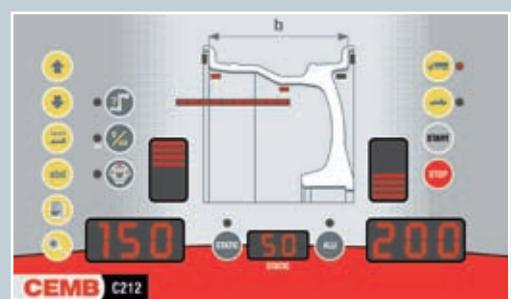
Light alloy rims, that are becoming more and more common on heavy vehicle wheels too, require the application of adhesive weights in 2 correction planes inside the rim, in hidden position. ALU "S" function allows to accurately set the dimensions (automatic distance and diameter) specific for the two correction planes.
